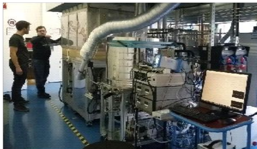
Fig. 3. ENEA gasification and EPFL/SP stack SOFC test rig
