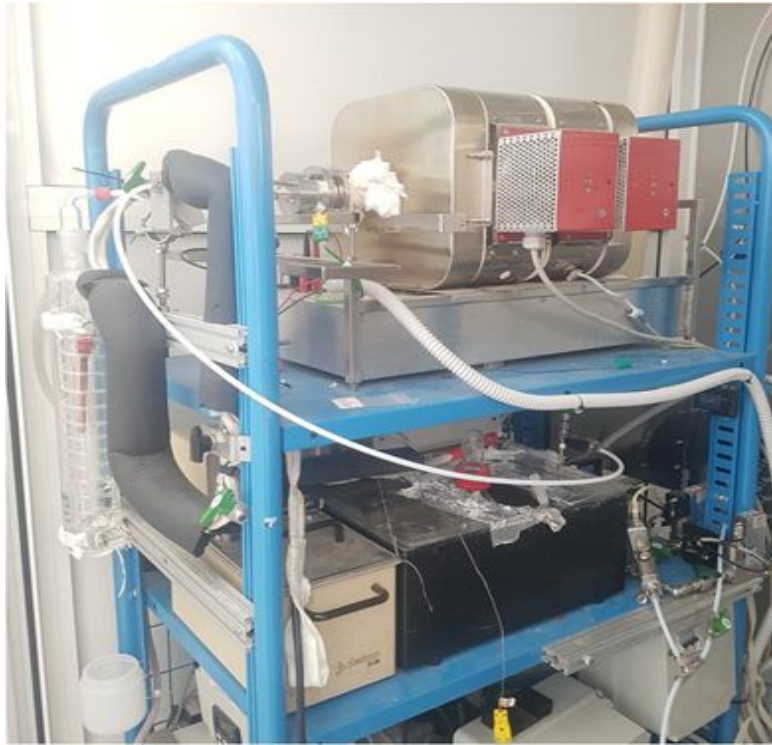
SOFC single cell test rig - gas and contaminants mixing stations (ENEA)
