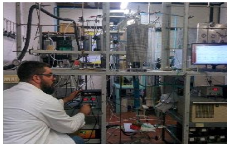
Fig. 2. UNITE gasification and UNIVAQ catalyst and sorbent test rig
