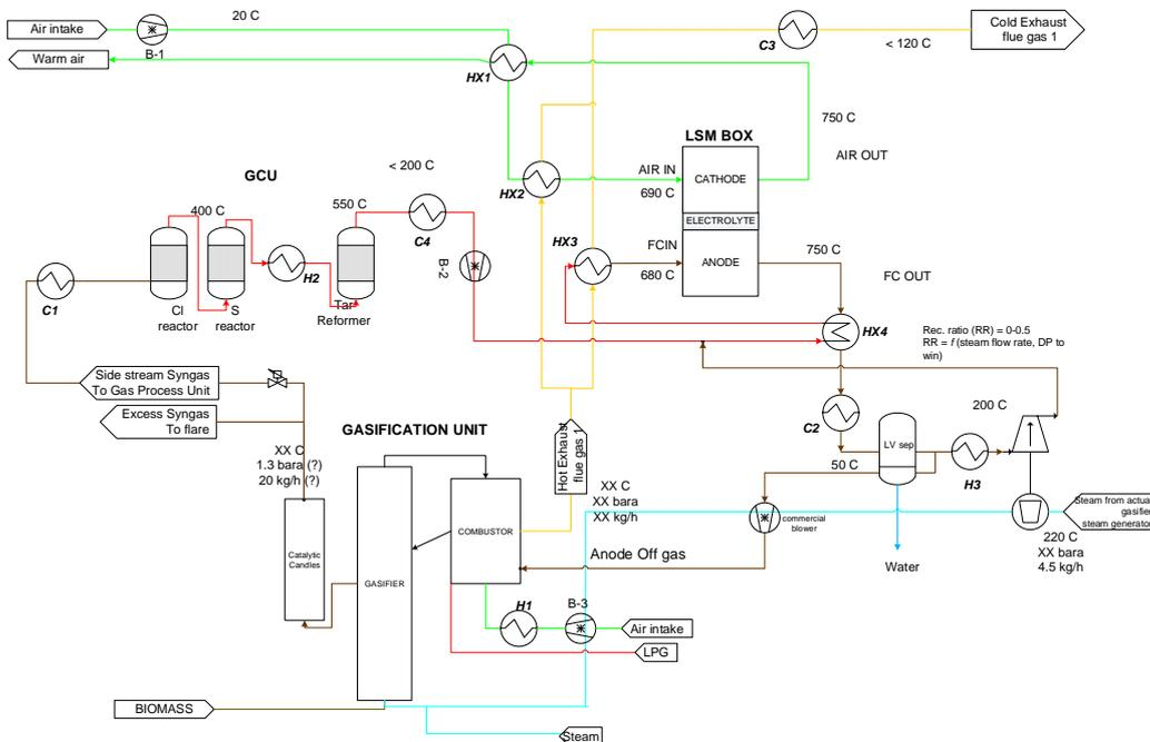
Figure 15. Option F process flow diagram of the BLAZE pilot plant. The AOG is sent to the SOFC LSM inlet stream (RR = 0.5) and the rest is burnt in the gasifier combustor. The recirculator condenses water before recycling. The gasifier is not compressed and the suction blower is placed after the GCU, after the cooler C4 (provided by HyGear, modified by EPFL LAMD and GEM). C: cooler; H: heater.
