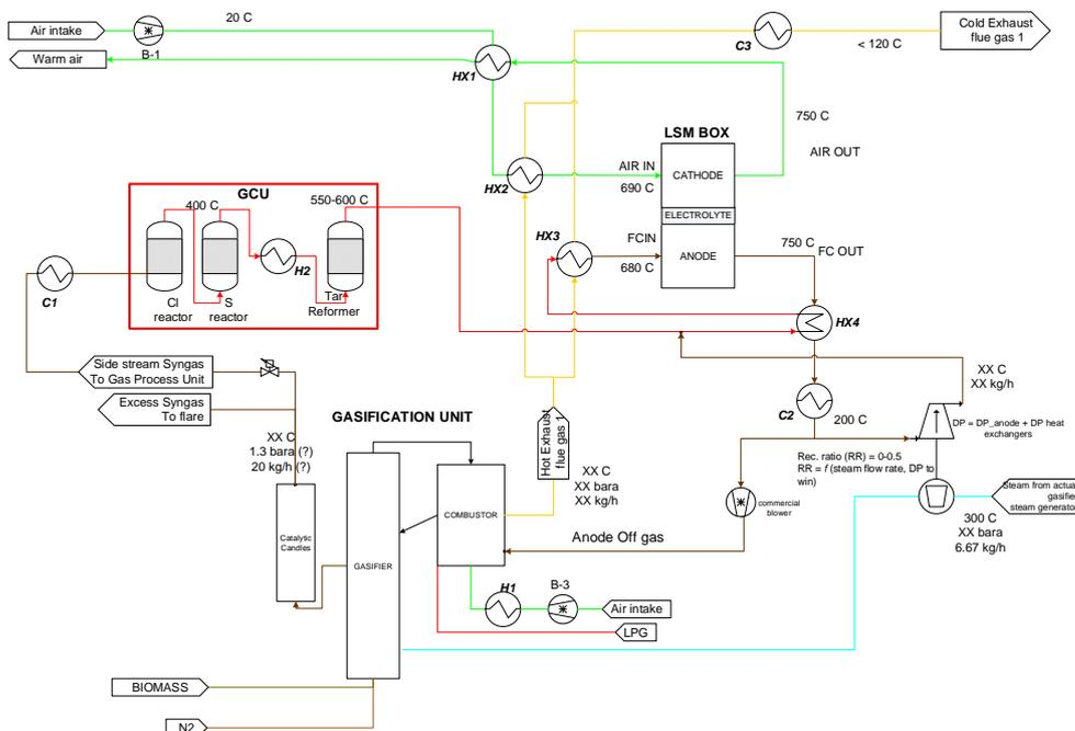
Figure 10. Option B process flow diagram of the BLAZE pilot plant, with a pressurised gasifier. Option F is analogous; instead of using a pressurised gasifier, it counts with a suction blower B2, after C1. The AOG is sent to the gasifier combustor and to the SOFC LSM inlet stream (RR = 0.5) (provided by HyGear, modified by EPFL LAMD). C: cooler; H: heater.
