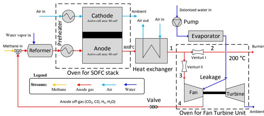
Figure 5. Recirculator integrated for a 6 kW<sub>e</sub> stack with natural gas as feedstock (provided by EPFL LAMD).
