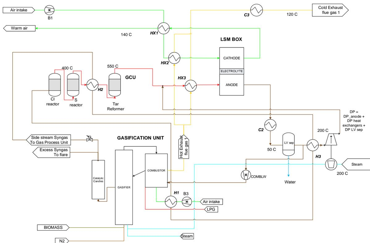
Figure 16. Option B process flow diagram of the BLAZE pilot plant. The AOG is sent to the SOFC LSM inlet stream (RR = 0.5) and the rest is burnt in the gasifier combustor, with heat exchange (same configuration for options D – Figure 14 and F – Figure 15; PFD F has moreover a cooler, C4, downstream the tar reformer) (provided by HyGear, modified by EPFL LAMD and GEM). C: cooler; H: heater.
