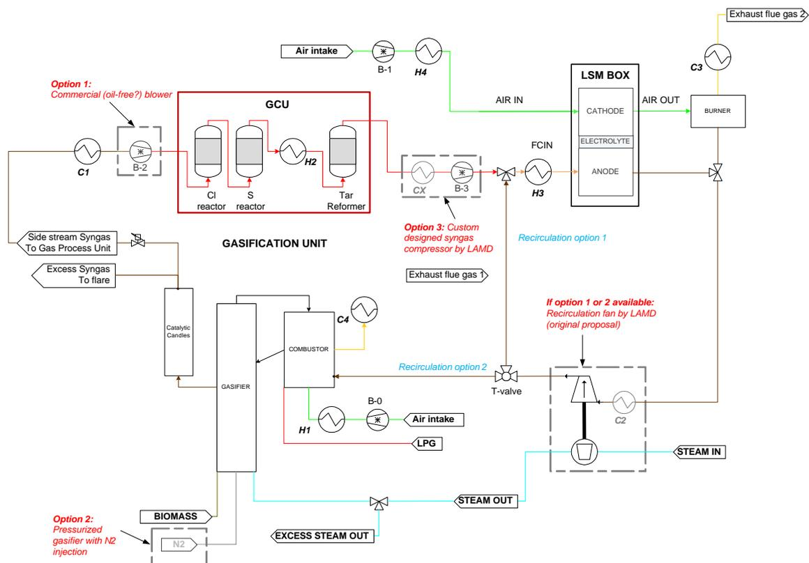
Figure 8. Process flow diagram of the BLAZE pilot plant, showing the recirculation options 1 and 2 and the possible custom designed compressor (option 3) (provided by HyGear, modified by EPFL LAMD). C: cooler; H: heater.
