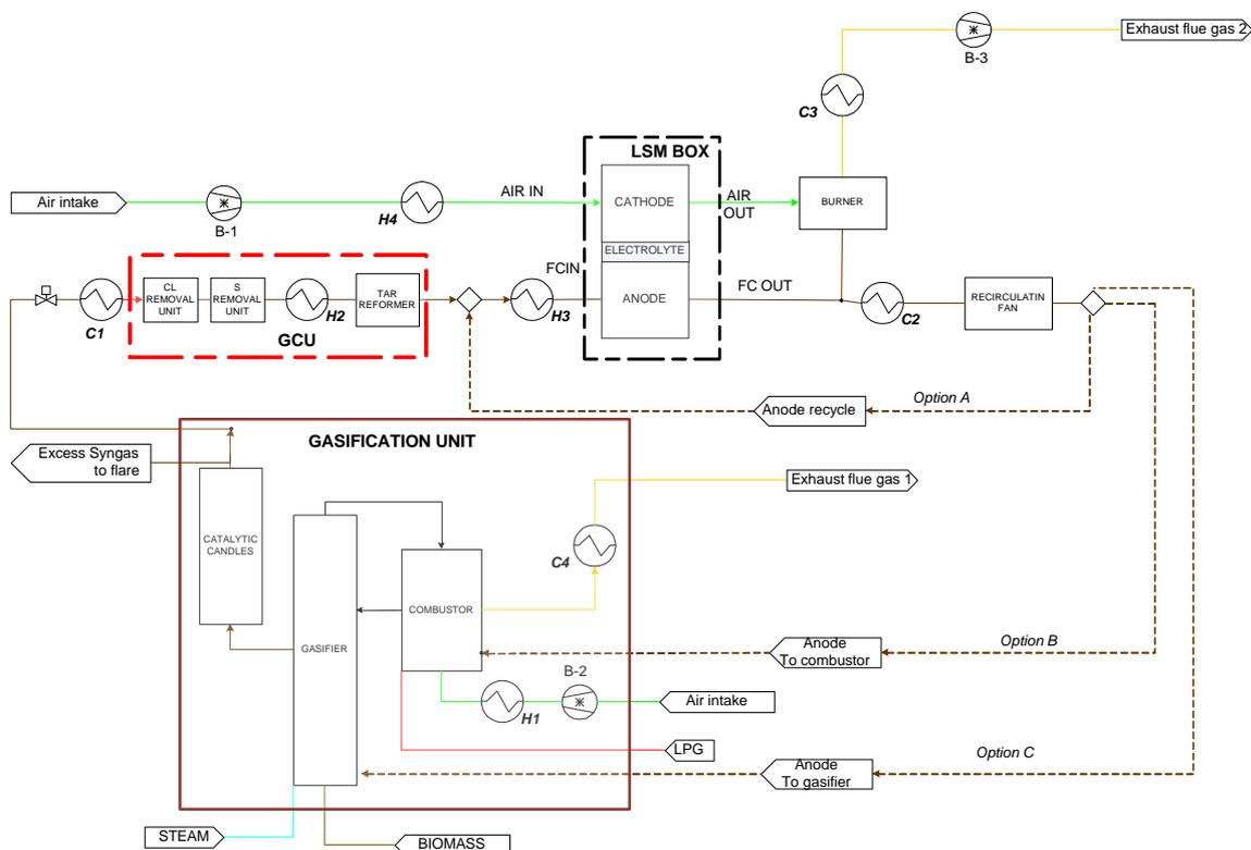
Figure 7. Process flow diagram of the BLAZE plant prototype system, showing the multiple recirculation options A, B and C (provided by HyGear, modified by EPFL GEM). C: cooler; H: heater.
