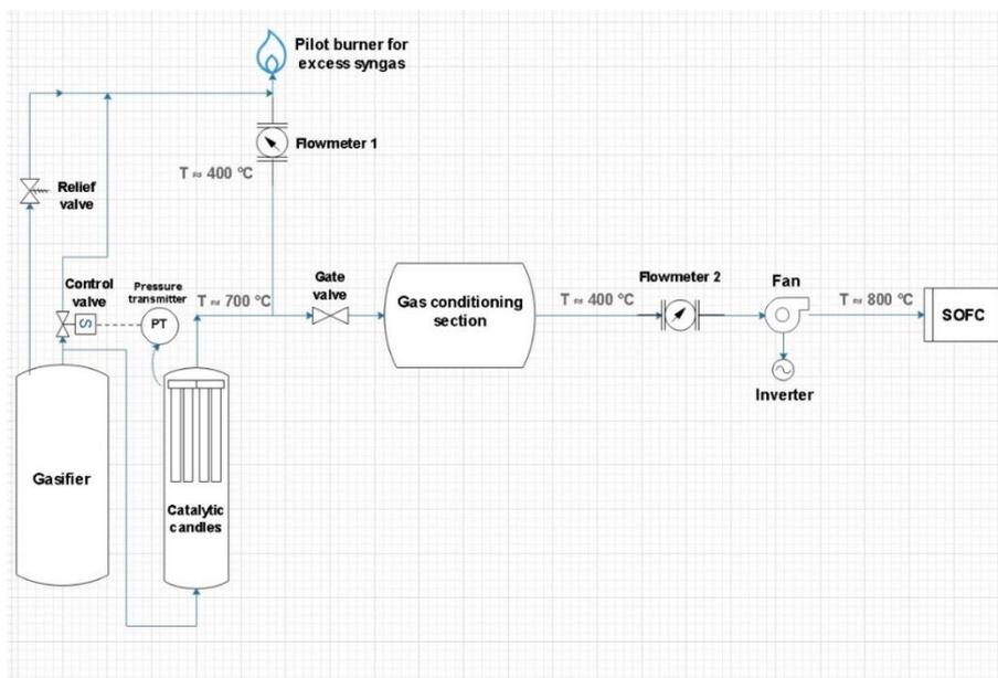
Figure 4. Detail of the syngas split (provided by USGM).
