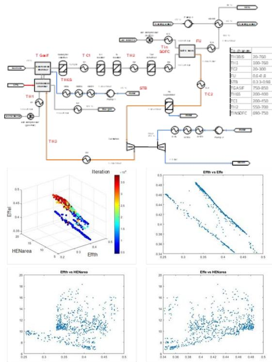
**Figure 10:** PFD proposed for optimization. In red: optimization variables (range of variation in the table) and Pareto front
