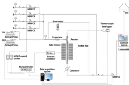
**Figure 4:** UNIVAQ Micro reactor test rig scheme
