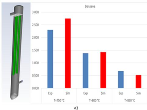
**Figure 8:** BLAZE modelling: benzene CFD simulations (mg/Nm<sup>3</sup>)
