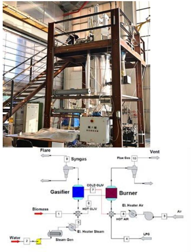
**Figure 11:** Pilot scale gasifier PFD and photo
