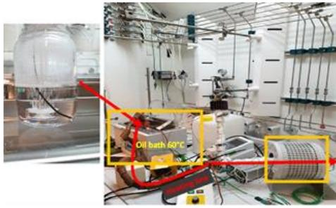
**Figure 7:** EPFL test-bench and modification for producing H<sub>2</sub>S from the decomposition of sulfolane
