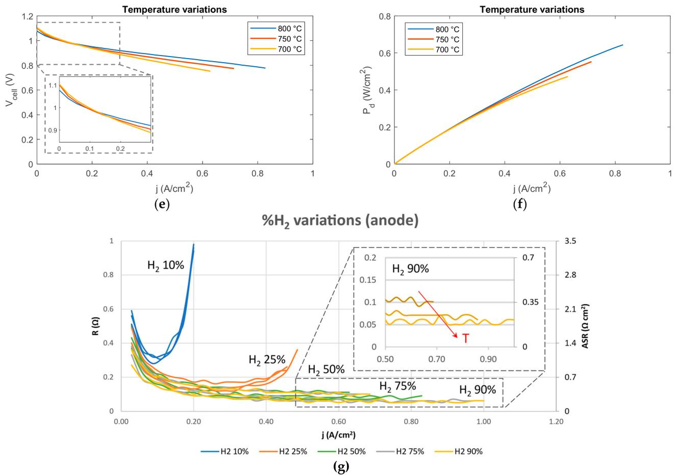
**Figure 6.** Experimental performance voltage & power curves: (a,b) H<sub>2</sub>%<sub>vol</sub> variations (T = 750 °C;  $\lambda$  = 1.4); (c,d)  $\lambda$  variations (T = 750 °C; H<sub>2</sub> 50%<sub>vol</sub>); (e,f) IV curve for T variations (H<sub>2</sub> 50%<sub>vol</sub>;  $\lambda$  = 1.4); (g) Resistance and Area Specific Resistance curve for H<sub>2</sub>%<sub>vol</sub> variations (T = 750 °C;  $\lambda$  = 1.4).
