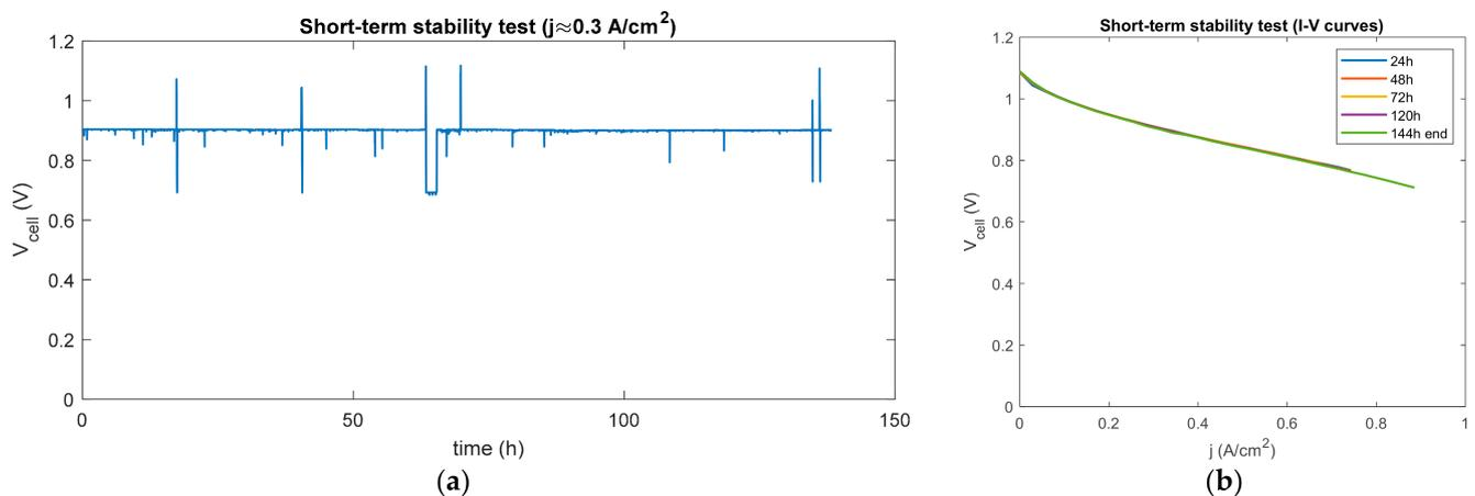
**Figure 8.** Experimental short-term stability test results: (a) cell voltage acquisition; (b) daily IV curves performed during the short-term test.
