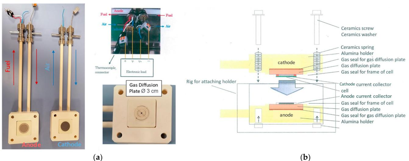
**Figure 4.** (a) All-Ceramic SOFC Test Holder used for the study; (b) schematization of cell assembly procedure.
