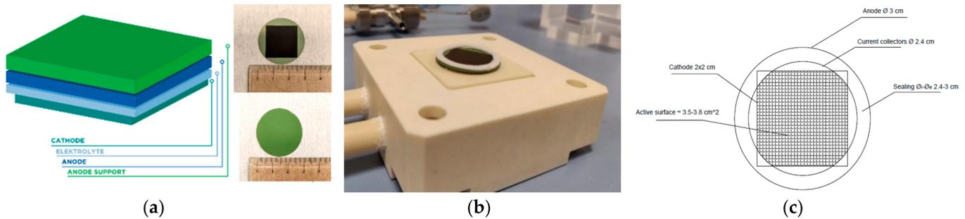
**Figure 5.** (a) Schematic and geometry of anode-supported SOFC (Ni-YSZ/YSZ/GDC-LSCF) (Ni-Yttria-Stabilized Zirconia/Yttria Stabilized Zirconia/Gadolinia Doped Ceria-Lanthanum Strontium Cobalt Ferrite) used; (b) button cell assembly in the holder; (c) Schematic of net active surface [49].
