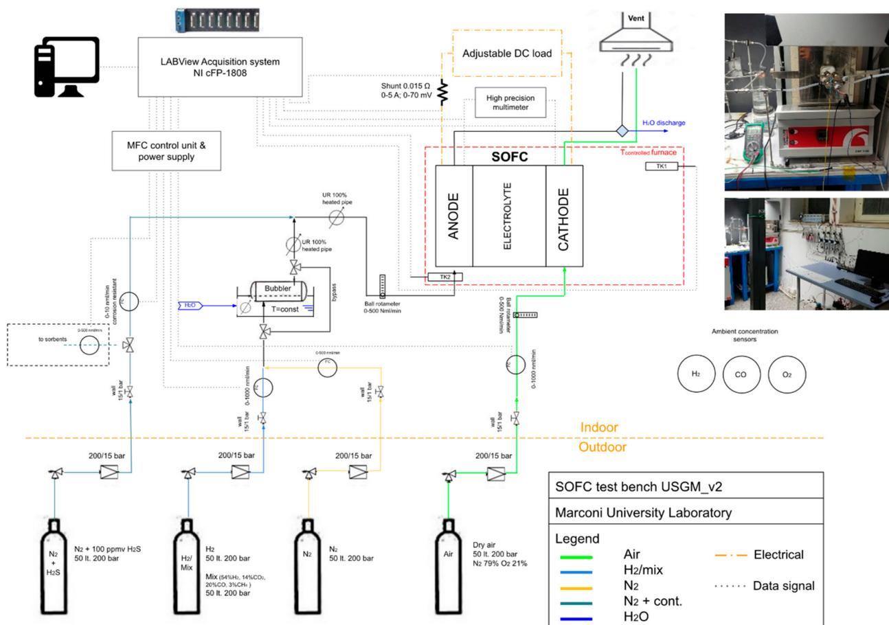
**Figure 3.** Experimental SOFC test bench setup scheme.
